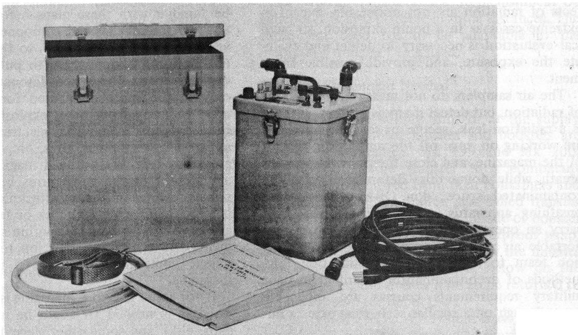
Figure 2-2.—IC/T2-PA portable radiation monitoring instrument with accessories.
